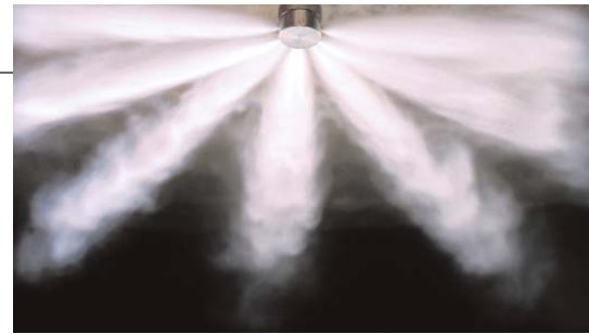
A clean agent, Novec 1230, is sprayed into the air at a 3M testing facility.
